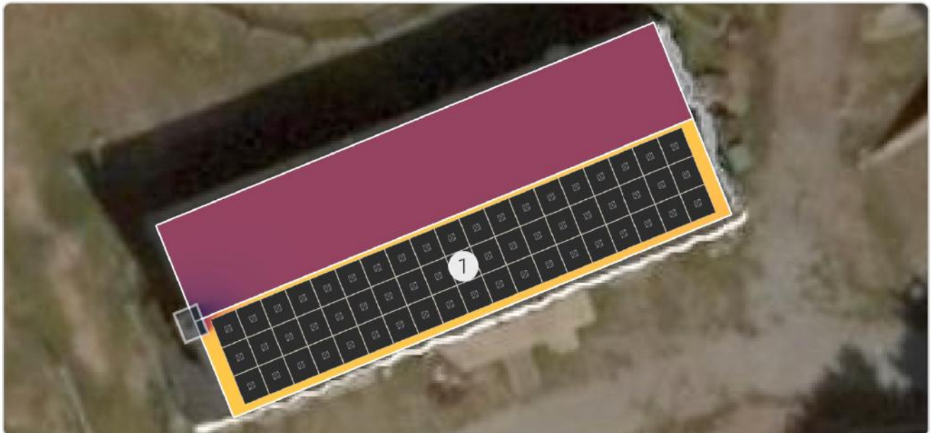
PHOTO 4 -LAYOUT OF SOLAR PANELS ON THE SQUASH HOUSE
